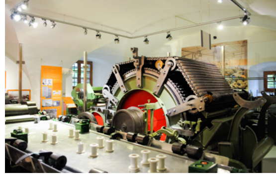
Old carding machine used to separate threads of material before spinning. Photo: Neža Renko.
