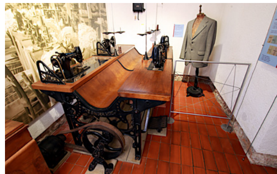
Commercial Singer sewing machines used in garment manufacturing trade. Photo: Jaka Blasutto.
