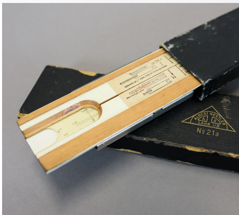
Used by engineers and engineering students to carry out quick and fairly accurate calculations, slide rules were a common tool in mechanical and electrical engineering, aircraft design, the military, in surveying, and in all other fields where logarithms, trigonometry, roots, squares, multiplication, and division were required. Slide rules were eventually replaced by the HP-35 calculator, which France Rode helped design in 1972. Technical Museum of Slovenia. Photo: Nebojša Tejić, STA.
