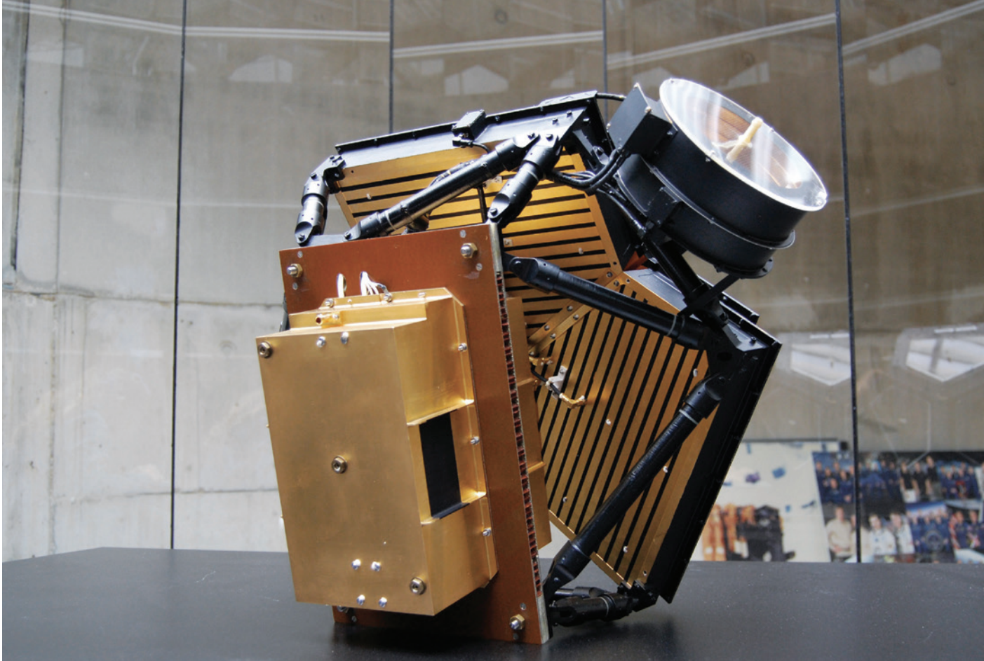
The plasma spectrometer for the Voyager space probe. Photo: KSEVT.
